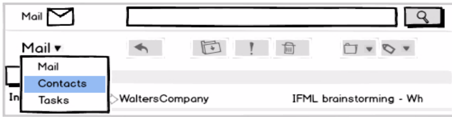
Figure A.4 - A menu allows one to switch from the MailMessages to the Contacts view components
