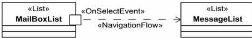
Figure 11.12 - Stereotyped UML diagram with IFML Extensions
