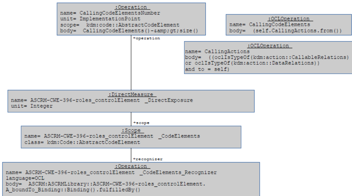
Figure 7.9 - ASCRM-CWE-396-roles-controlElement role direct exposure computation with SMM OCLOperations, Operation, DirectMeasure, Scope, and Recognizer
